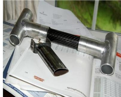
together with wing demount and overnight tethering. Consideration is being given to material changes to aid weight reduction with the use of carbon and self-jigging to aid assembly. Sample parts are under test. A design review will be undertaken when we have a better understanding of the components we need to carry and the adjustments felt necessary.
