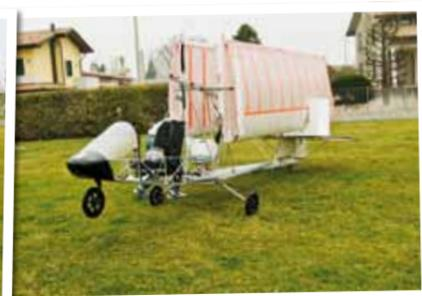
**Rigging and de-rigging the NCWS Minifox is a simple one-person job and, wings-folded, the aircraft is only 2.3m wide, tucking easily into the corner of a shed**
