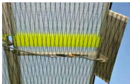
**Above: proper aeroplane features include an elevator trimmer**
