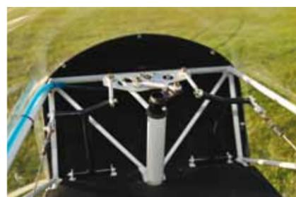
Clever: the rudder pedals are interconnected and the nosewheel steered by a common bellcrank
