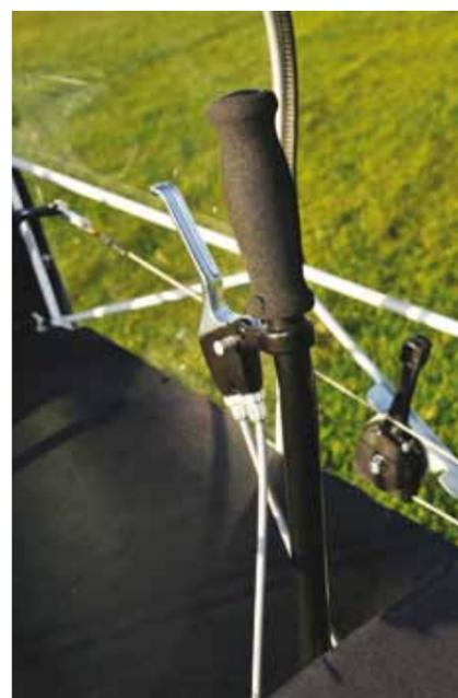
Wheel brakes are operated by a lever on the stick
