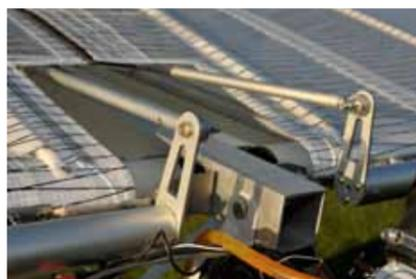
**Below: further good design – the ailerons are operated by rods and torque tubes**
